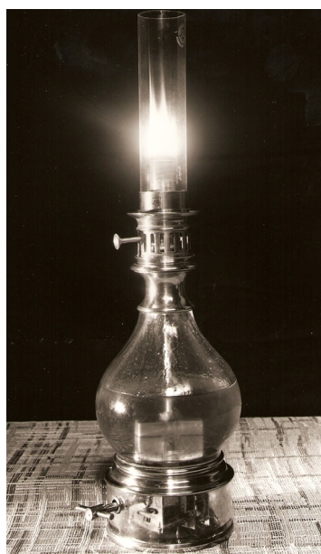
Pumped lamp. Oil is forced up to the burner by the clockwork driven pump in the base.
