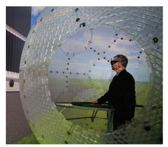
Fig. 2 - Spherical walk simulator inside the BigCAVE (photo: Dorota Patschull).
