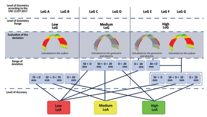
Fig. 3 – Evaluation of geometric reliability in terms of deviation between the point cloud and the model. Depending on the LoG of the element analysed, the deviation is evaluated on the entire surface, on the generatrixes and directrixes, or on both, according to different ranges.
