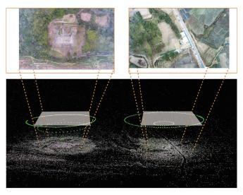
Fig. 5 - Point cloud map of circular flight.
