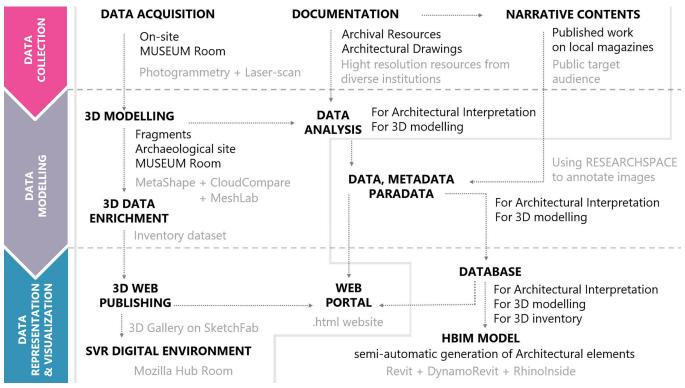
Fig. 2 - Methodological Workflow for the creation of a digital ecosystem, including processes and software.
