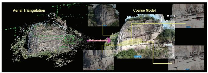
Fig. 9 - Coarse Model Results of the Baiyun Temple Site Based on the Nap-of-the-Object Photogrammetry Data.
