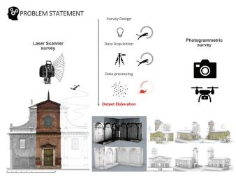
Fig. 3 – Digital survey pipeline.
