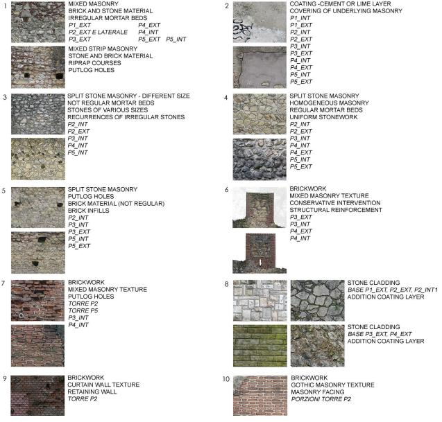
Fig. 9 – List of constructions types based on materials (stone, brick, mortar, and cladding) found on the defined masonry, taking archaeological stratification as a comparison.
