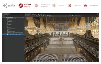
Fig. 13 – Importing main hall models within the Game Engine Unity platform and acoustic processing using the Steam Audio plugin.
