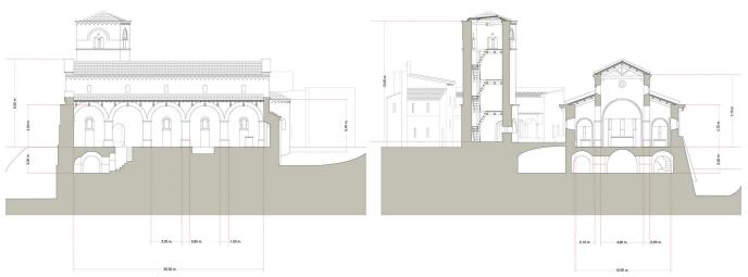
Fig.17 - Virtual reconstruction of the medieval fortified complex of Satrianum. Longitudinal section (A-A') and cross section (B-B') of the Cathedral, extracted from the three-dimensional virtual model. Elaboration by M. Tricarico.
