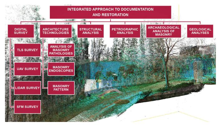
Fig. 8 – Methodology used for the project to define the conservation and restoration of the wall portion carried out in collaboration with the University of Florence and the University of Siena.
