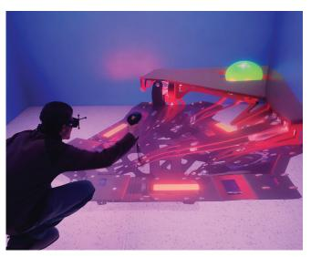
Fig. 10 - Virtual prototype of the Stewart platform – BigCAVE.
