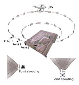
Fig. 4 - Flight schematic of the drone in point-of-interest surround mode.
