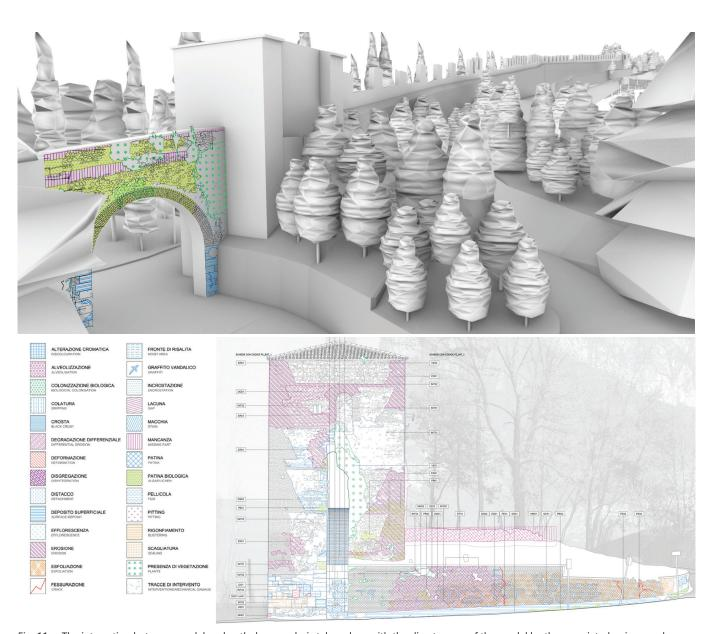
Fig. 11 – The interaction between model and pathology analysis takes place with the direct query of the model by the associated unique code. Georeferencing is possible through the use of the TLS cloud with GPS points as a basis for three-dimensional modelling.
