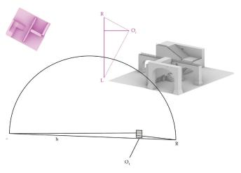
Fig. 13 – Floor plan (in purple) and axonometric view of the 3D model with the perspective setting and position of the projection centre related to the architecture (graphic elaborations by the author).
