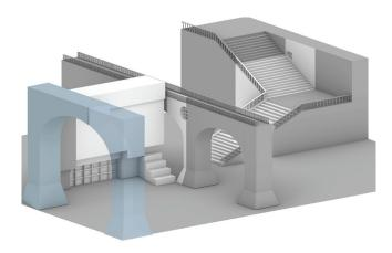
Fig. 14 – Axonometric view of the 3D model with the reconstructive hypothesis in which the colours indicate the level of reliability: the elements deduced from the etching in light grey, the altered elements in blue, the hypothesised elements in dark grey, the omitted elements in transparent blue (graphic elaboration by the author).
