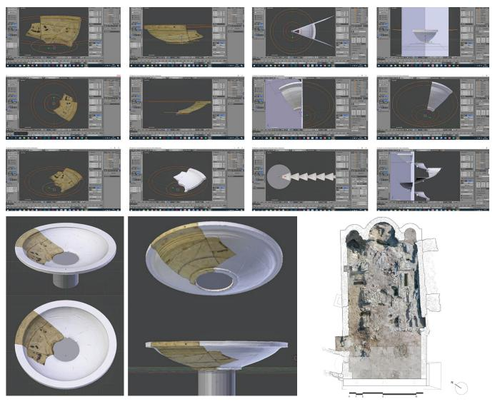
Fig. 12 - The different stages of three-dimensional reconstruction of the Karabournaki plate in its integral form. From the photogrammetric model of the real object to the virtual model. Screen extracts from Blender 3D, processed by Margherita Tricarico.
