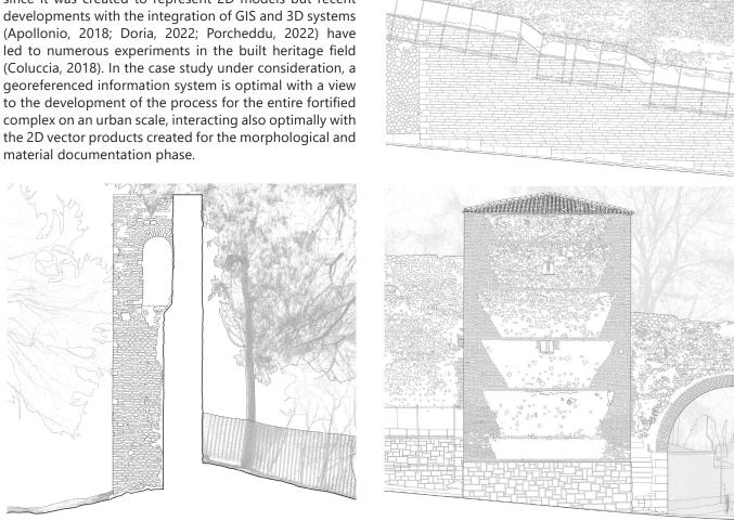
Fig. 6 – Two-dimensional vector drawings made from TLS point clouds. The drawings produced were used by the entire research team as support for the analysis and diagnostic phase.
