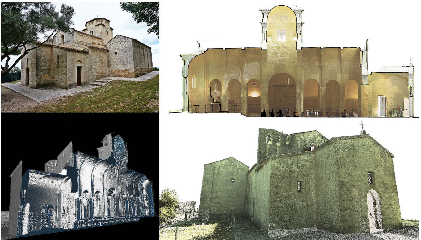
Fig. 1 - Survey data of Santa Maria of Portonovo: the TLS point cloud in several views.
