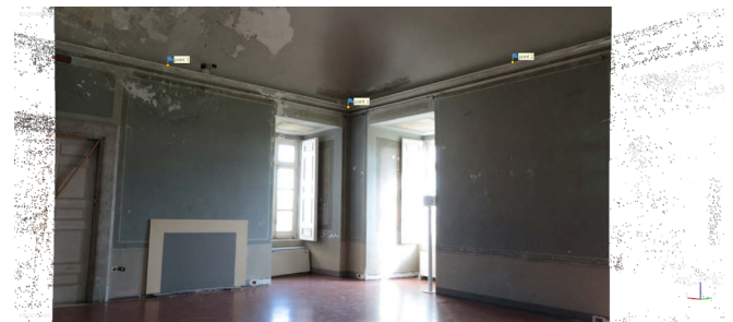
Fig. 10 - Point cloud of the Real Sito di Carditello produced with Structure from Motion process using images taken by a drone.
