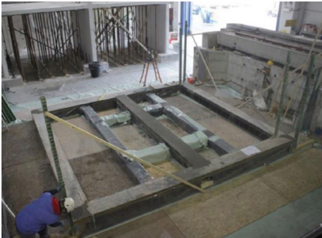
Fig. 2 Building prototype construction site within the EUCENTRE laboratories in Pavia. The structure was built directly above the shaking platform.
