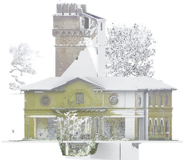
(Above) Fig. 6 The Mill of the Cantone, state of fact; (below) Fig. 7 The Mill, point clouds+nurbs model.
