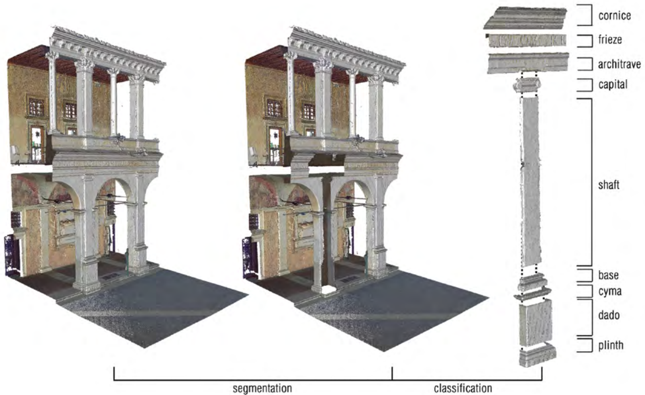
Fig. 4 - Point cloud segmentation and classification process
