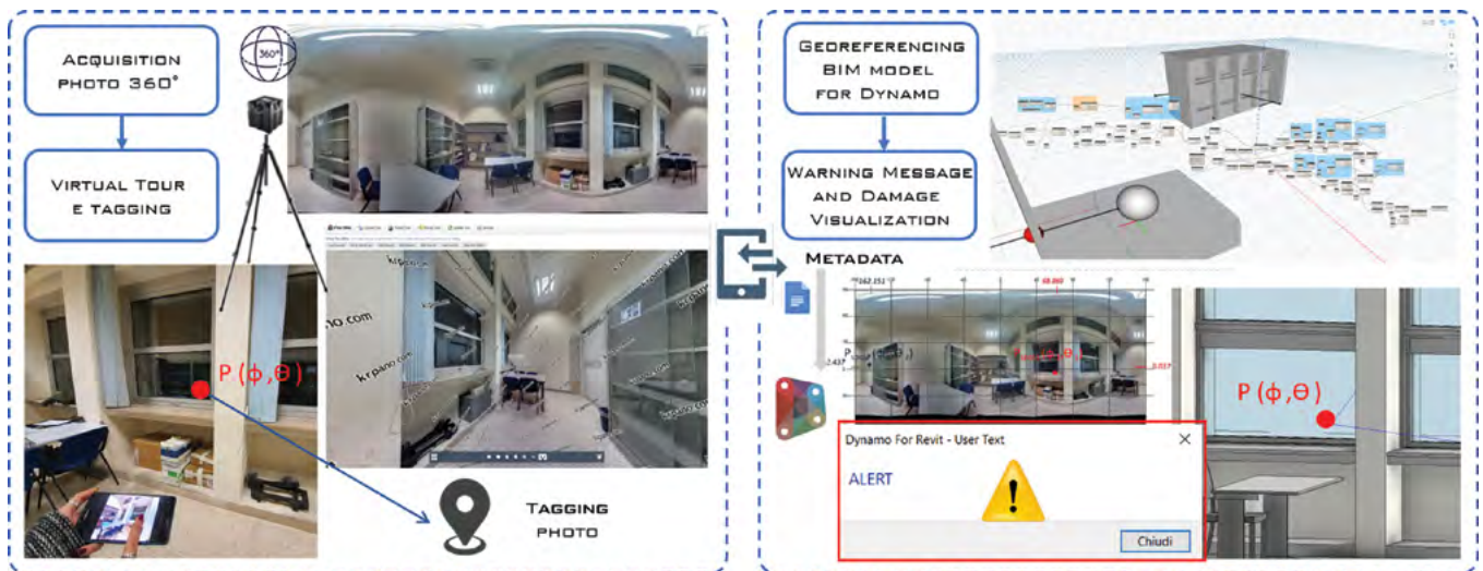
Fig. 1 - Synthesis of the digital process that relates data acquired in the real world with information tagging on spherical images, linking them to metadata through their geo-references within the BIM model itself.
