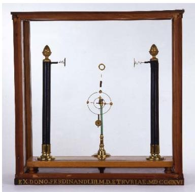
**Fig. 1.** Electromotive perpetual pendulum dated 1816. By courtesy of Physics Collection of Scientific Instruments, Department of Physical Sciences, Earth and Environment, University of Siena.
