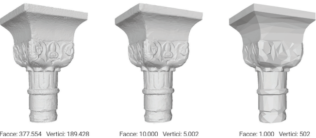
Fig. 4 - On the left, optimization of the mesh for a capital of the Southern Pavilion, realized with SfM methods from 3D Eye rods. Some views of the capitals of the Northern Pavilion and of the Southern Pavilion, realized as mesh 3D models, and optimized in the number of polygons. Each capital and architectural-decorative element is associated with identification codes that allow to associate an information sheet with each element. Below, NURBS modeling of the Palazzo complex, based on Rhinoceros software, and the texturing phase on Cinema 4D software.
