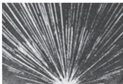
**Fig. 1.** Particle tracks in a Wilson’s cloud chamber
