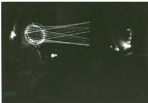
Fig. 1. One of our Herriott delay lines: the envelope of the laser beams, made visible by Moden’s pipe smoke, describes a hyperboloid.
