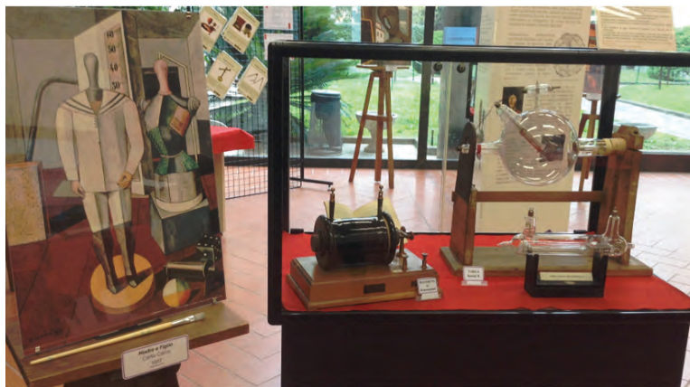
Fig. 5. Carrà picture matched to the instruments related to X-rays: a Ruhmkorff coil (close to the detail of the picture that recalls it) and the X-rays tube
