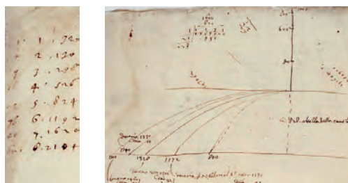
Fig. 2. Left: data about the odd numbers law. Gal72. Detail of folio 107v. Right: the measures of the ranges of the projectile motion with horizontal initial velocity. Manuscript Gal 72. Detail of folio 116v (with kind permission of Biblioteca Nazionale Centrale di Firenze ).
