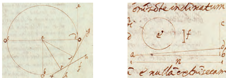
Fig. 1. Left: proofing of the upward force necessary to balance the effect of gravity along an inclined plane. Manuscript Gal 71. Detail of folio 95r. Right: by decreasing the slope of the plane ad until the horizon, the sphere e , if subject only to its weight f and to no resistance, can be moved by a force less than any given force. Manuscript Gal 71. Detail of folio 97r (with kind permission of Biblioteca Nazionale Centrale di Firenze ).
