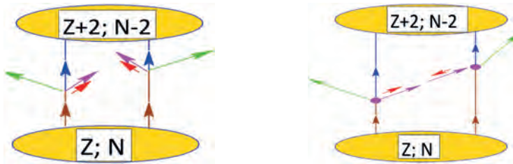
Fig. 2. Left: two-neutrino double beta decay represents two simultaneous single beta decays and cannot distinguish between Majorana and Dirac neutrinos. This decay is allowed for Dirac and Majorana neutrinos. Right: neutrinoless double beta decay is only possible for massive Majorana neutrinos. For a finite mass, helicity is not a good quantum number and at the left vertex an antineutrino is emitted while it is absorbed at the right vertex as neutrino (only possible for Majorana neutrinos). In order not to be helicity forbidden by the spin direction, the exchanged neutrino must have a mass. So, the detection of the neutrinoless double beta decay would show the Majorana character of the neutrino.
